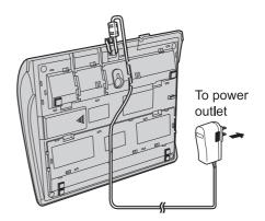
3 Dress the telephone line cord as shown. Tuck the telephone line cord inside the wall mounting adaptor, then push it in the direction of the arrows (1) and (2).
